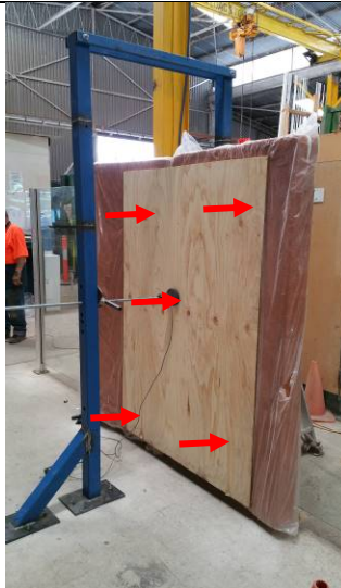
Photo 6 Infill Horizontal Loading – Wind Loading
