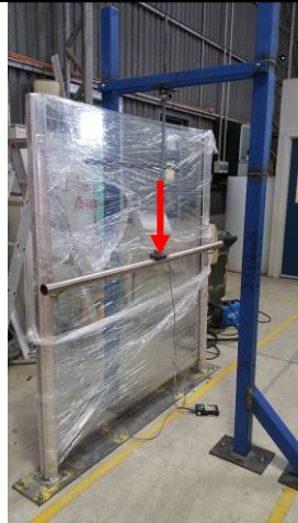
Photo 12 Hand Rail Loading Outwards & Downwards - Welded to Stainless Steel Bracket
