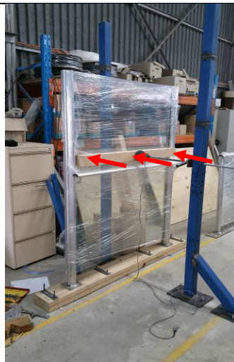
Photo 10 Horizontal Loading – Timber Fixed
