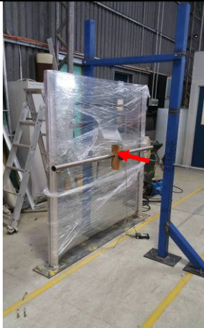
Photo 12 Hand Rail Loading Outwards & Downwards - Welded to Stainless Steel Bracket
