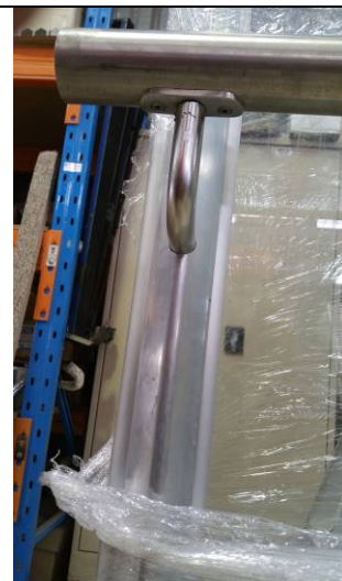
Photo 13 Hand Rail Loading Outwards & Downwards – Riveted to Stainless Steel Bracket
