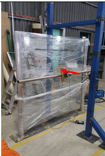
Photo 13 Hand Rail Loading Outwards & Downwards – Riveted to Stainless Steel Bracket
