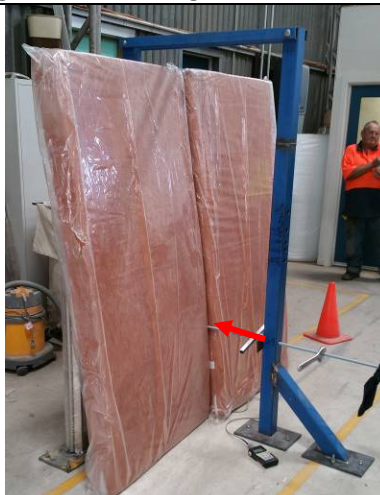
Photo 6 Infill Horizontal Loading – Wind Loading
