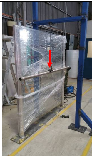
Photo 13 Hand Rail Loading Outwards & Downwards – Riveted to Stainless Steel Bracket
